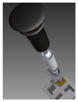
Pre-warmed incoming air (supply) is channelled naturally via an existing chimney void and enters the room either through the fireplace opening (with minimal alteration) or a low level vent. No electrical connections and no fans or heaters are required.
