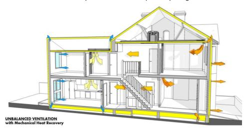
Warm air is forced out through cracks and cavities while cold air is sucked in at the other end of the house. In comparison Ventive saves time, money and effort. With no operating costs, no maintenance costs and no forced heat loss you get the right solution from day one and no hidden extras. As shown below, house that is passively ventilated by Ventive suffers no forced heat loss:
